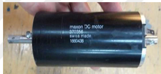
Figure 4.13. DC motor graphite brushed Maxon RE50 Ø50 mm
