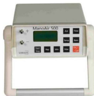
Figure 4.8. Micromanometer device type ManoAir 500
