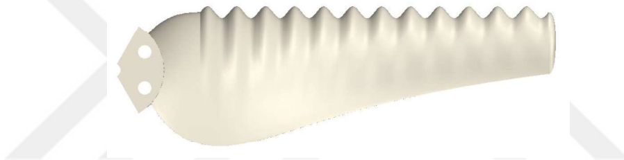
Figure 1.18. The leading edge tubercles technique modele implemented on the blade (present study)
