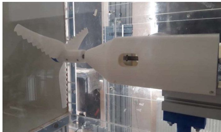
Figure 4.11. Wind turbine placed in the test section
