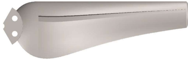
Figure 1.21. The vortex cavity implemented on the upper surface of the blade (present study)
