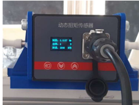
Figure 4.12. The digital torque and tachometer sensor DYN-200
