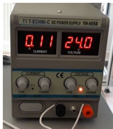
Figure 4.17. DC power supply (TT T-ECHNI-C YH-605D)
