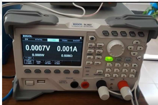
Figure 4.16. Electronic load unit (Rigol DL3021 Precision)
