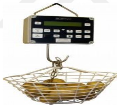
Figure 3.1. Martin Lishmans's digital potato hydrometer (PW2050) used to measure specific gravity and dry matter content of potato crop
