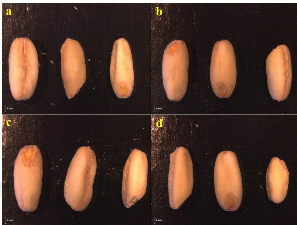
Figure 5.3. Coating and volume differences between inert dusts at 2000 ppm: (a) halloysite, (b) bentonite (c) sepiolite and (d) zeolite
