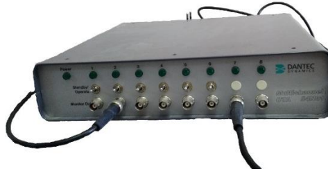
Fotoğraf 2.3. DANTEC multichannel 54N81 model hot-wire anemometresi
