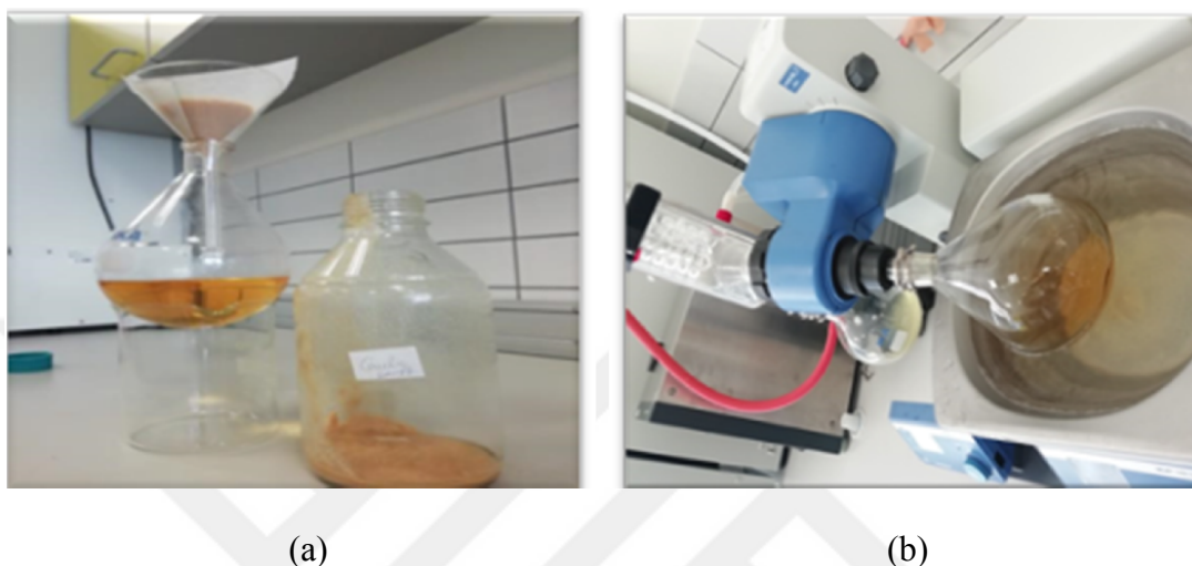
Figure 3.4. The process of filtering the garlic powder extract by filter paper (a) and evaporating the ethanol from garlic powder extracts (b)
