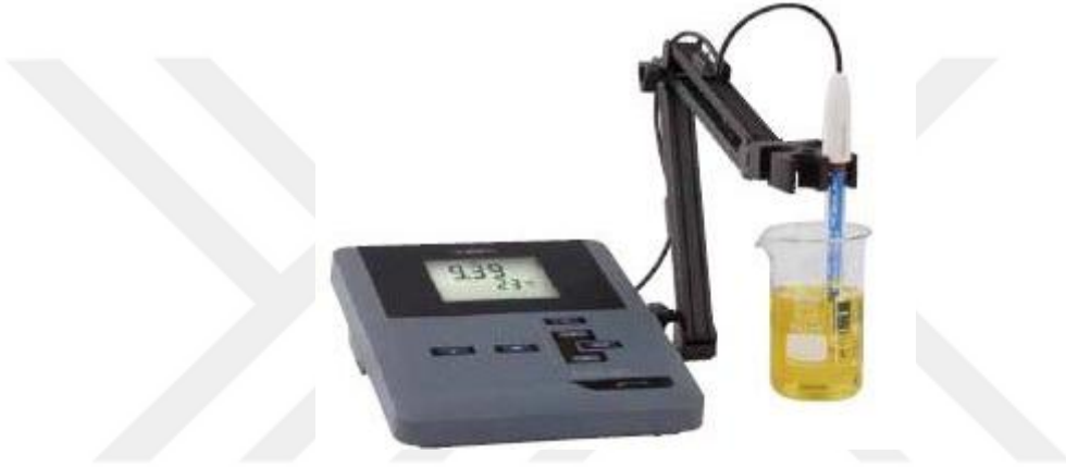
Şekil 3.1. pH Metre (Inolab pH 7110 set 2 (pH 720))
