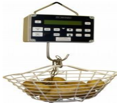
Figure 3.1. Martin Lishmans's digital potato hydrometer (PW2050) was used to measure specific gravity and dry matter content of potato tubers
