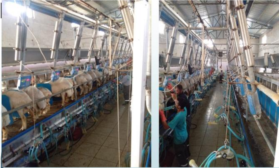
Figure 3.1. Fullwood milking parlor 2x48 for sheep of MeMuTa Dairy Sheep Farm at Niğde
