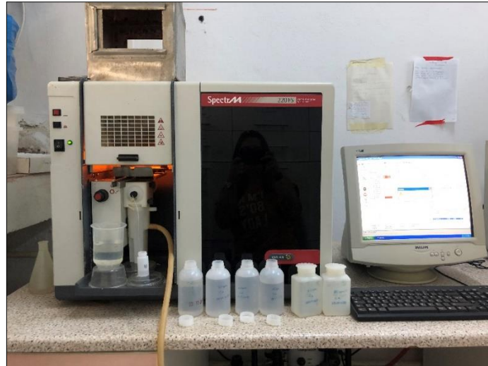
Figure 2.17. Atomic absorption spectrophotometry
