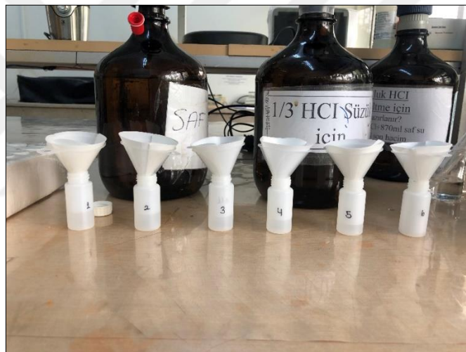
Figure 2.16. Filtering samples dissolved in HCL solution
