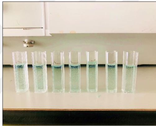
Figure 2.6. Samples for the measurement of FRAP values through a spectrophotometric absorbance at 593 nm
