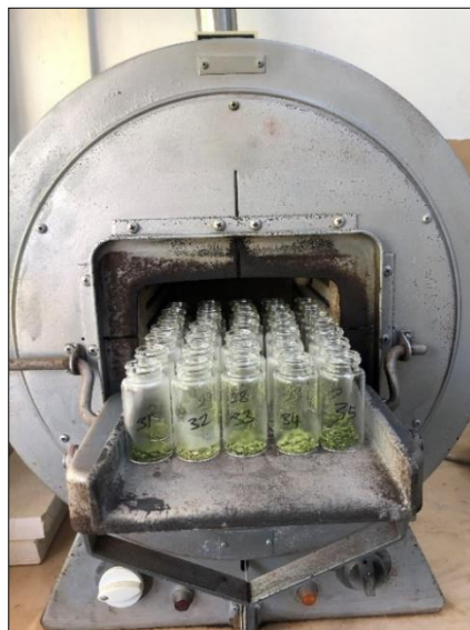
Figure 2.14. Placement of samples into the ashing oven
